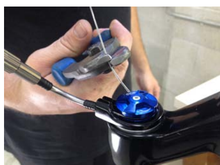
11. Cut cable and install cable end.
