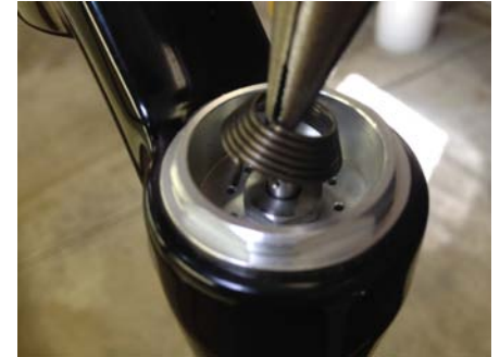
3. Take spring from remote lockout kit and set end of spring in a hole roughly 180 degrees opposite from the hole on the adjuster shaft.
