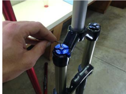
2. Remove lockout knob with 1.5mm allen.
