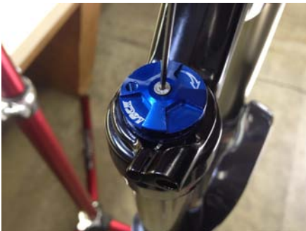
7. Install top cap so that cable stop is 90 degrees from cable exit.
