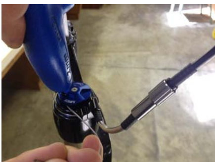
10. Tension cable and tighten set screw.
