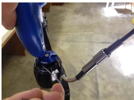
10. Tension cable and tighten set screw.
