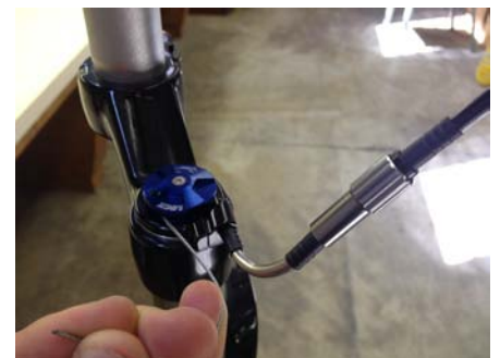
9. Cut housing to size then install barrel adjuster and cable guide.
