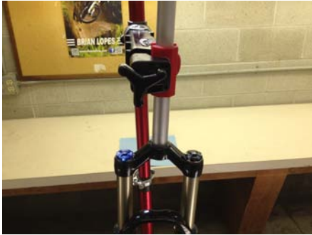
1. Make sure fork is upright for install.
