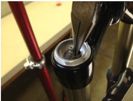
4. Tension by twisting and installing in hole 180 degrees from starting hole.
