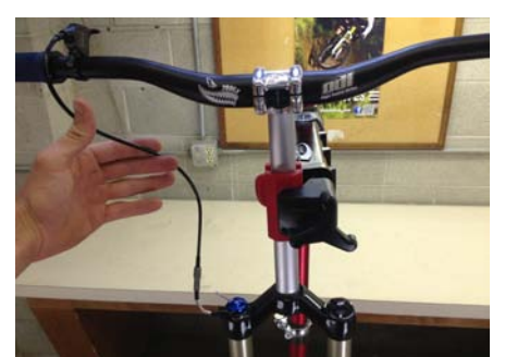
12. Make sure everything is secure and working properly. If remote is not opening from lock then you need to go back to step 4 and add tension.
