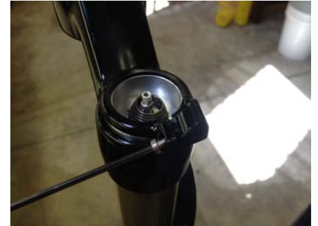
6. Install cable guide so that cable will exit sideways.
