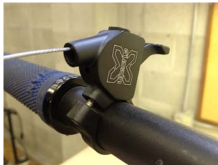
8. Install remote on handlebars.
