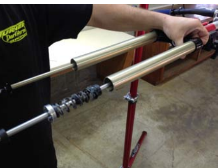
12. Reinstall air spring system.
