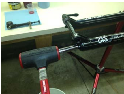
5. Use softblow to break seal between footnut and lower leg.
