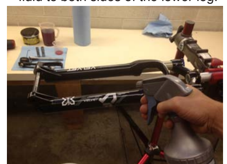
19. Clean with alcohol and clean towel/rag. Then reinstall on bike and go shred!
