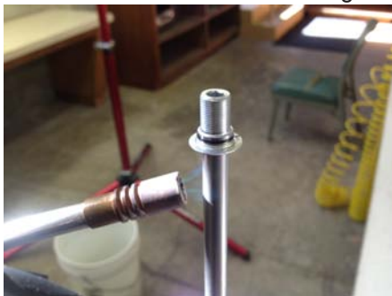
8. Clamp in vice with 9mm shaft clamps then put heat to shaft below footnut.
