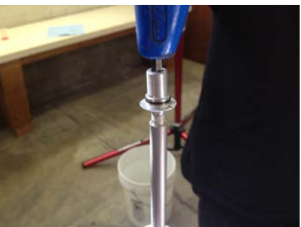
9. Remove footnut with 6mm allen wrench.
