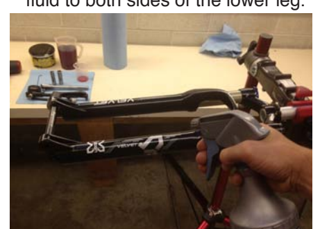
13. Clean with alcohol and clean towel/rag. Then reinstall on bike and go shred!
