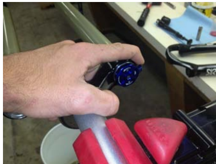
8. Lock fork out before reinstall.
