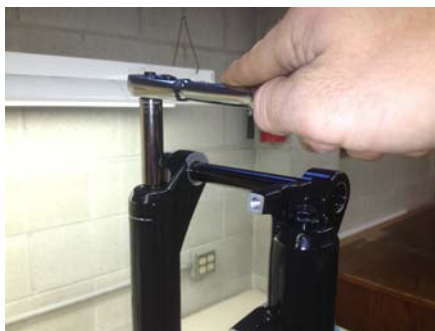
11. Reinstall footnuts and rebound knob.
