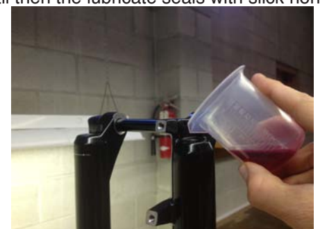
10. Add 15cc's of 7.5 Wt. suspension fluid to both sides of the lower leg.
