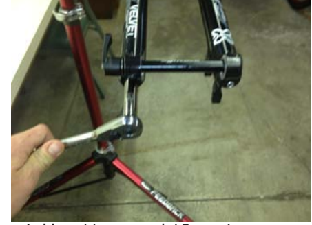
4. Use 11mm and 12mm to remove footnuts 50% of their threads.
