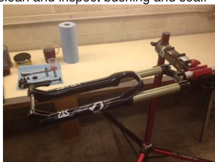
9. Reinstall lowers part way and flip vertically.
