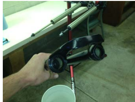
6. Remove lower and let drain while you clean and inspect bushing and seal.
