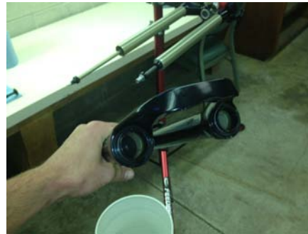
6. Remove lower and let drain while you clean and inspect bushing and seal.
