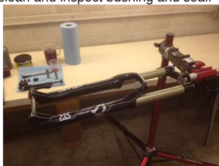
9. Reinstall lowers part way and flip vertically.
