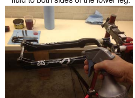
13. Clean with alcohol and clean towel/rag. Then reinstall on bike and go shred!
