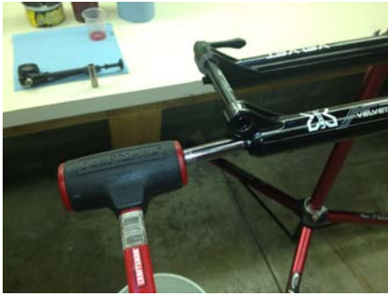
5. Use softblow to break seal between footnut and lower leg.
