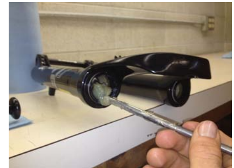
7. After removing and cleaning the foam ring, reinstall then the lubricate seals with slick honey.
