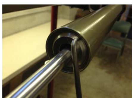
12. Reinstall rod and C-clip. Make sure C-clip is 100% seated in the groove.
