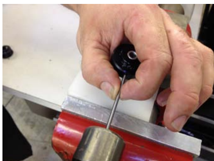
10. Line up your punch and tap the push-pin through the travel stop just far enough so that the stop can move freely.
